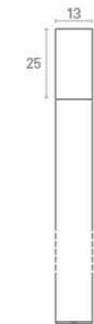
CLICK ZIP TWIN profile W 13cm x 2 (25cm combined) max. W up to cm 480
