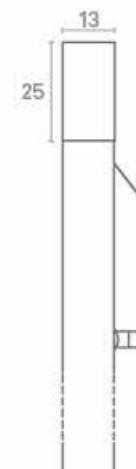
CLICK ZIP TWIN BG profile W 13cm x 2 (25cm combined) max. W up to cm 480
