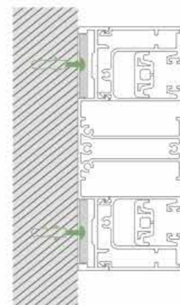
2. mounted cassette box in the reveal – the guides do not support it
