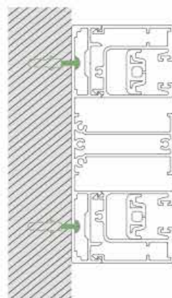
1. mounted to be self-supported by its guides
